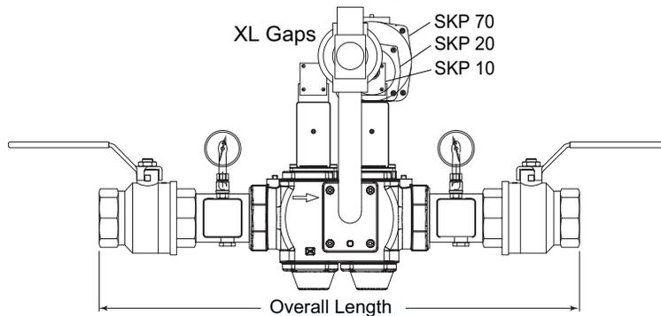
When using the Siemens SKP20 and SKP70 actuators for pressure regulating and ratio regulating functions, the sensing piping is not included. For proper operation, the sensing pipe should be at least 1/4" ID and connected a minimum of 5 pipe diameters downstream in a non-turbulent area.
